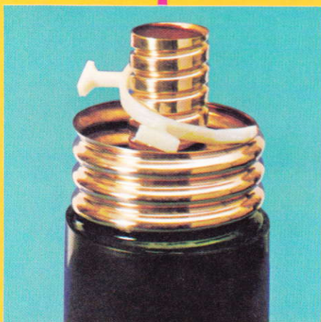
RF coaxial cable with helix spaced insulation and corrugated copper tube. This cable is suitable for use as an antenna feeder for outlet powers of up to 500 kW.
