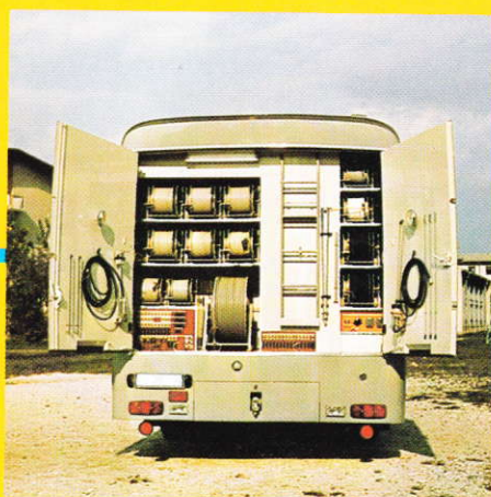
All transmission and power cables are accommodated on drums in the rear of the van, ready for connecting.
